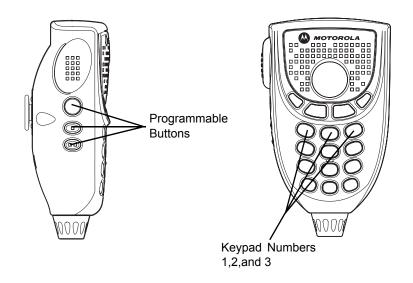
**Note:** Keypad numbers 1, 2 and 3 require the Preset Zone and Channel Enable field in the CPS to be enabled. Please check with a qualified radio technician to set them as **Mode Select** buttons.
